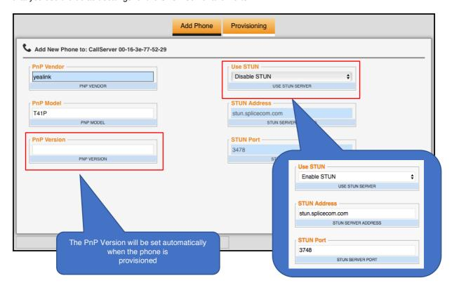
For Auto provisioning to work correctly you will have to set the PnP model Description to the correct type, if this is not set correctly then the phone may not work as you expect
